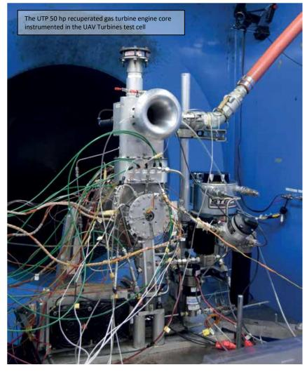
"Gas turbines work on the principle that the speed at the tips of the turbine blades is extremely high. In the case of a small turbine, that implies a shaft speed of 100,000-plus rpm, and how do you reduce that to a 6000 rpm propeller speed? You need a gearbox of some kind, and that takes you out of the model aircraft arena. That gearbox is itself a significant challenge.
